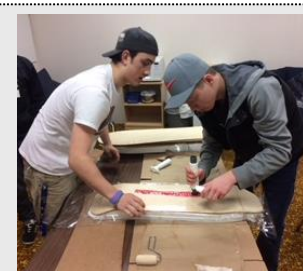
After students choose a design for their skateboard, a vacuum seal bag is used to press the board.
